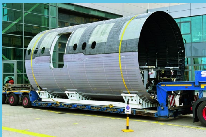
▲ Airbus' multi-functional fuselage demonstrator is a showcase for Victrex LMPAEEK™ based composites, with a fuselage structure being manufactured based on our materials (image courtesy of Airbus).
